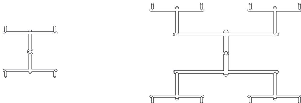
**FIG. 1:** Above are examples of 4-cavity and 8-cavity runner systems. While the exact cavity spacing layout and subsequent runner size is very dependent on part geometry, you can see the 8-cavity runner size is more than twice that of the 4-cavity runner. In this particular example, the 8-cavity runner size was 2.75 times the size of the 4-cavity.
