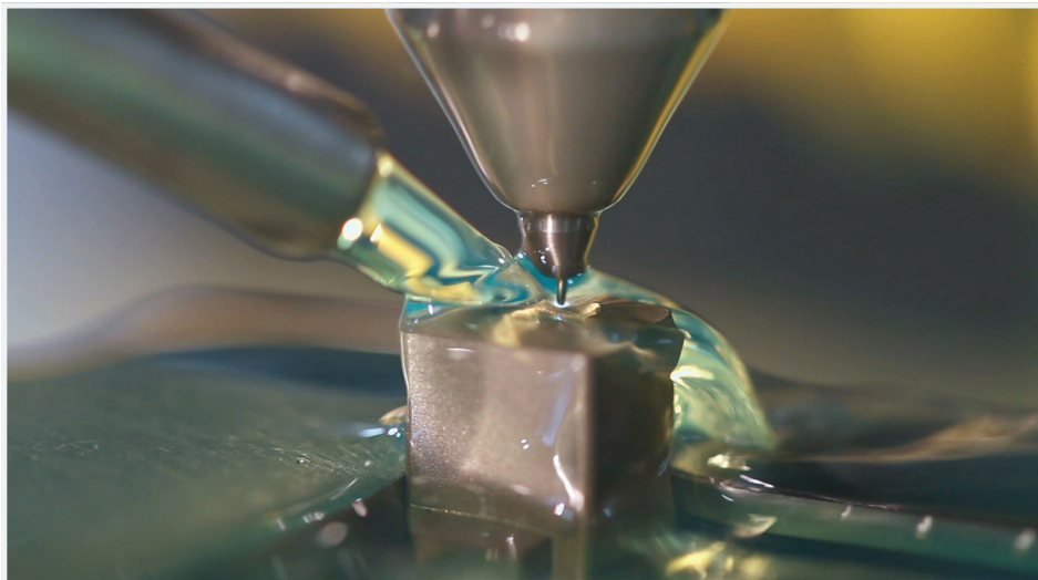
Sarix 3D EDM milling technology in action. MTD has the only Sarix machine in the U.S. being utilized for creating micro mold inserts.
