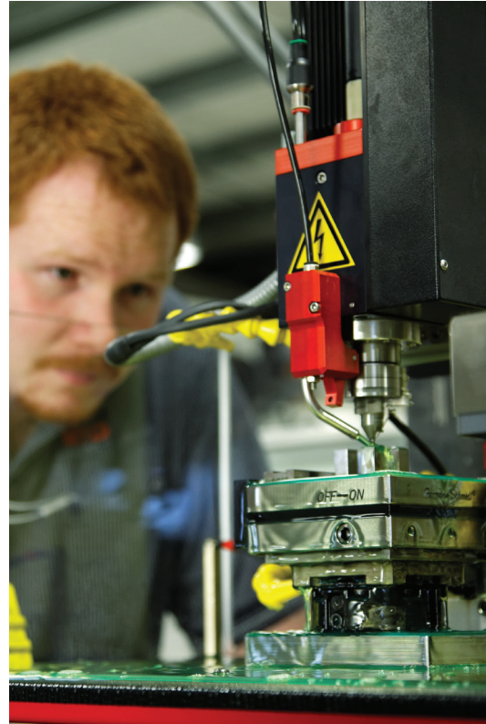
FIG. 3: Micromolding is impossible without an extremely precise tool. And molds with certain geometries are not possible without a Sarix 3D micro EDM milling machine.
