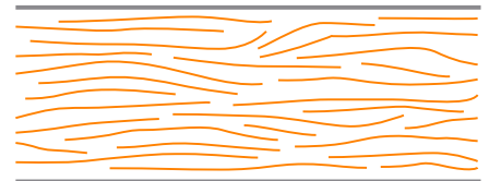
FIGURE 4: Polymer chains become aligned during the injection molding process.
